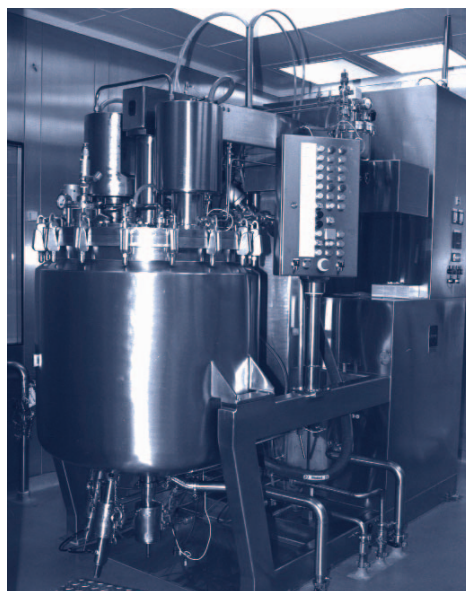
The homogeniser FRYMA VME 400 is part of the suspensions and liquid dosage equipment at the product manufacturing facility
